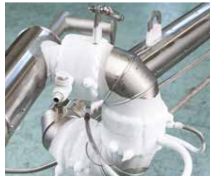
Cryoload swivels under load during FAT
