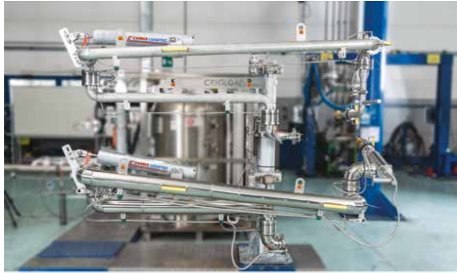
Cryoload twin bottom loading arms for use on LNG loading or unloading during FAT
