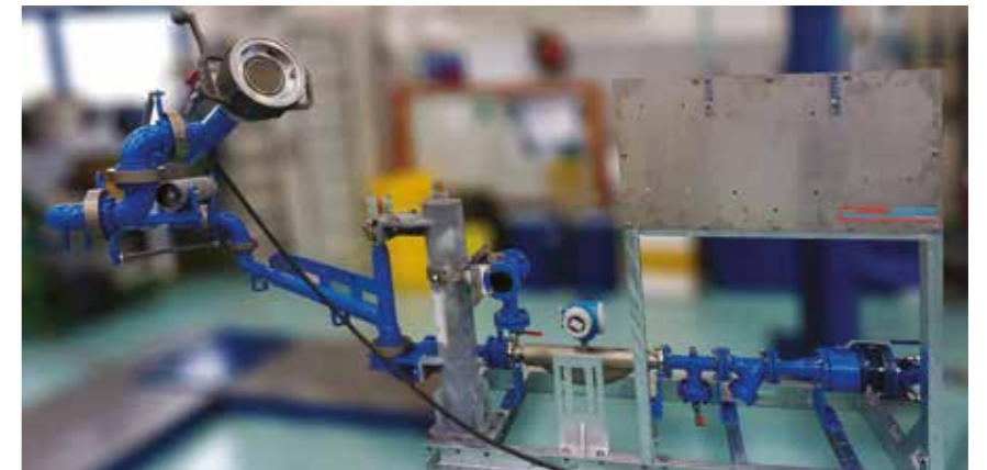
Bottom loading skid with meter, filter and controller - UK - Renewable Fuels industry
