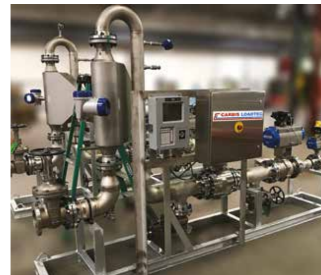
UAN, batch control, loading skid with connection to terminal automation system
