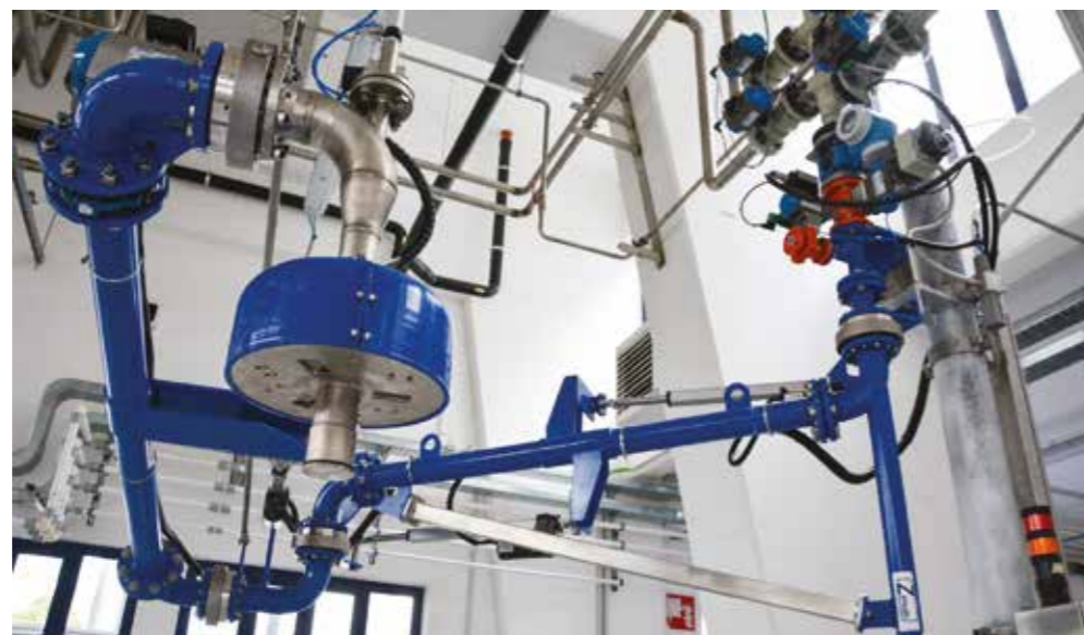
Autoload® PTFE lined IBC loading arm, electrically actuated with control valves and Titanium Drop pipe with anti-drip valve for clean loading. - Italy - Chemical industry
