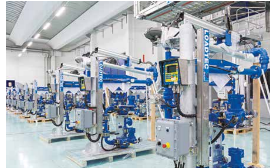
20 x Top loading skids with duty and standby metering system with batch controllers - Bangladesh - Fuels Industry
