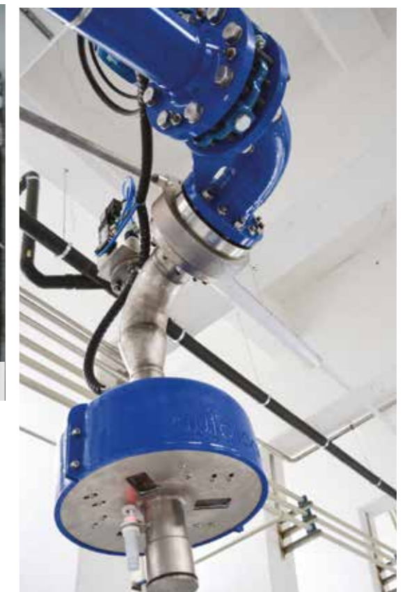
3D Printed Cone with multiple sensors for control and positioning of the Autoload® arm
