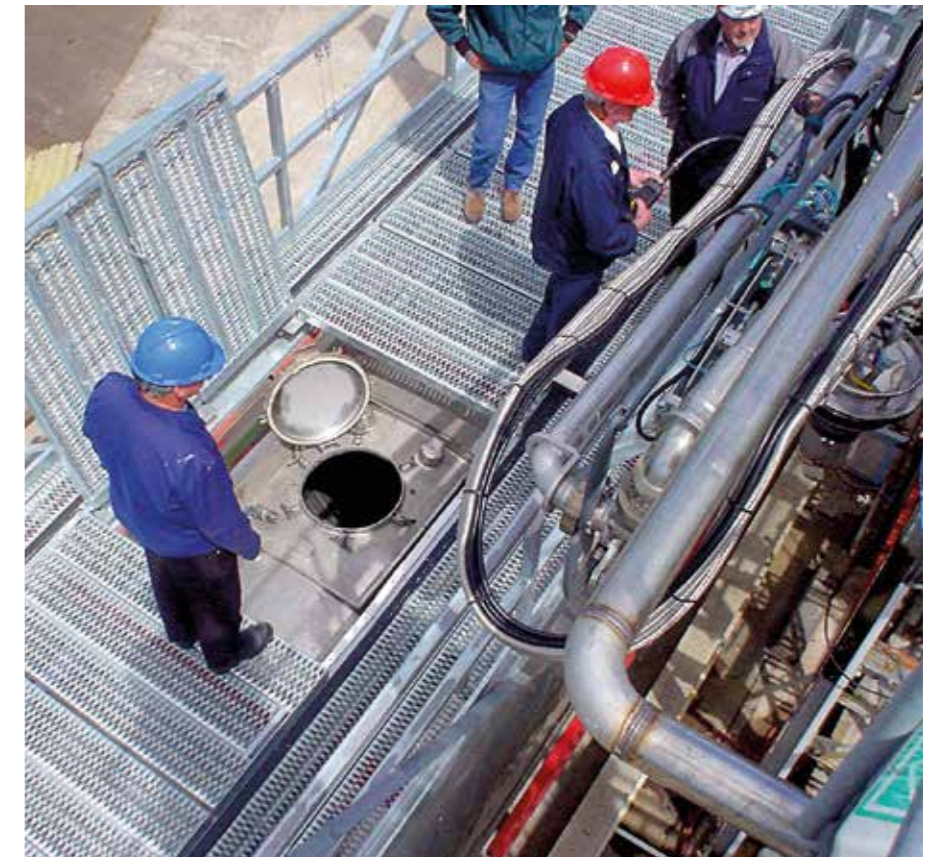
10m Hydraulic VELP with wide flip up panels providing access to tanker manlid - UK - Chemical Industry
