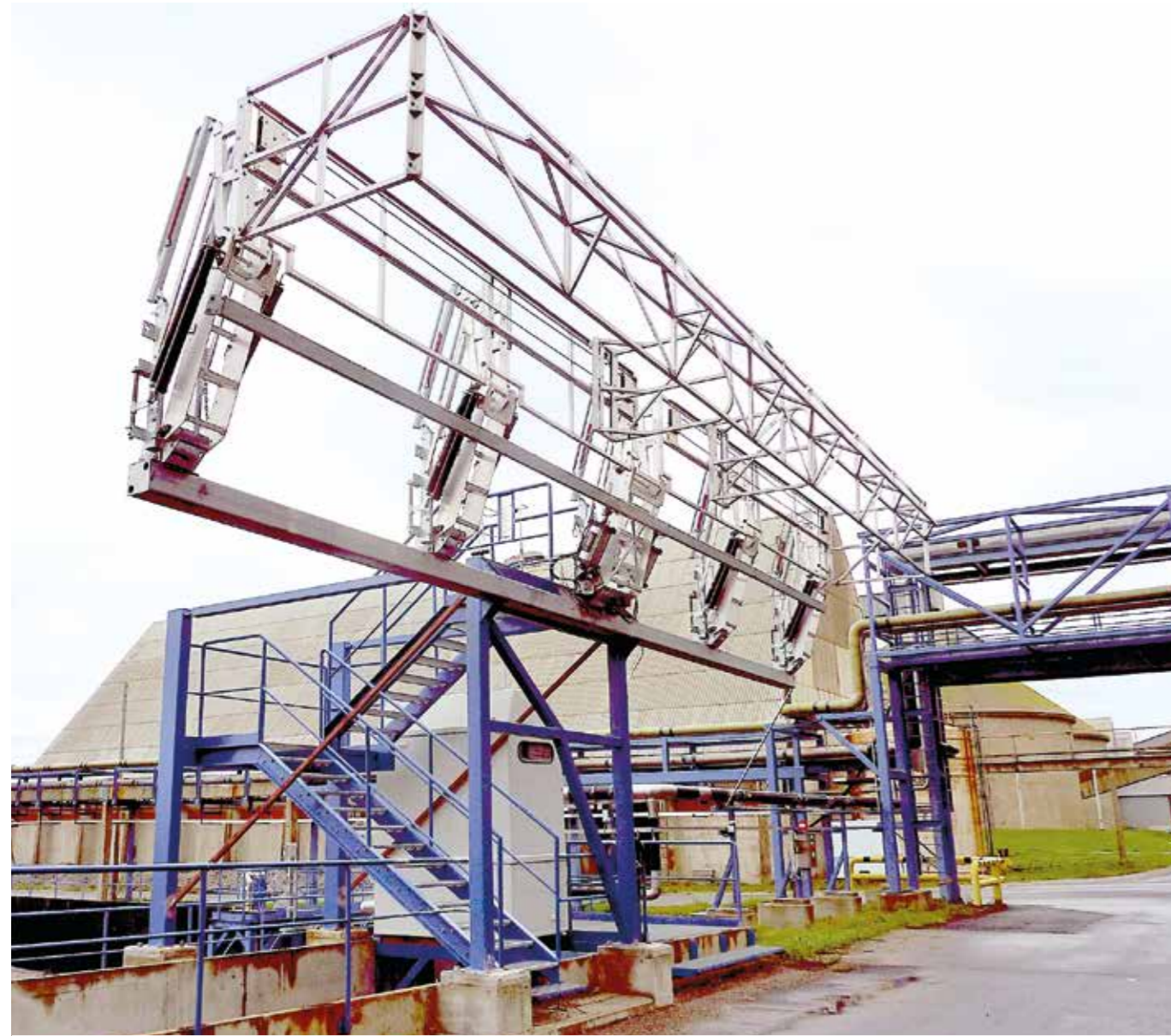
12m Large cage with internal tracking gate to reduce working area, all pneumatically operated - Finland - Fertiliser industry
