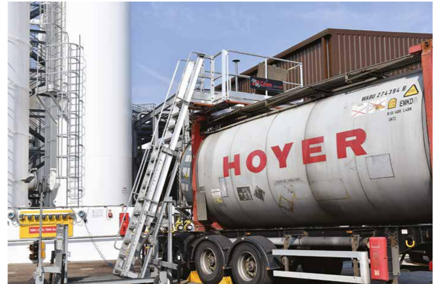
TC-10 Mobile Access Cart providing safe access to the top of an ISO container for venting during unloading - UK - Chemical Industry
