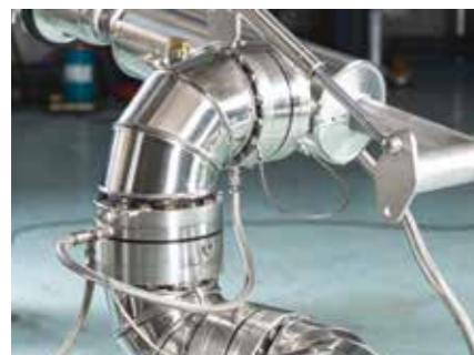
Cryoload swivels after testing
