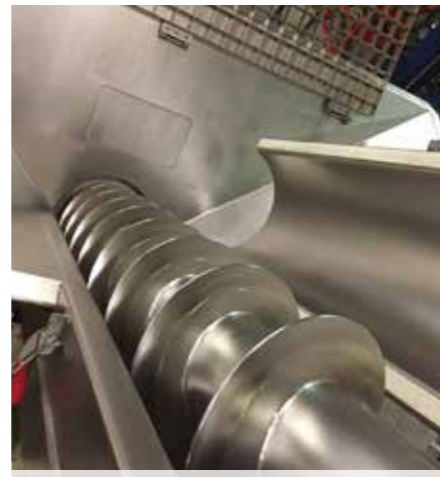
Automatic transportation via the screw
