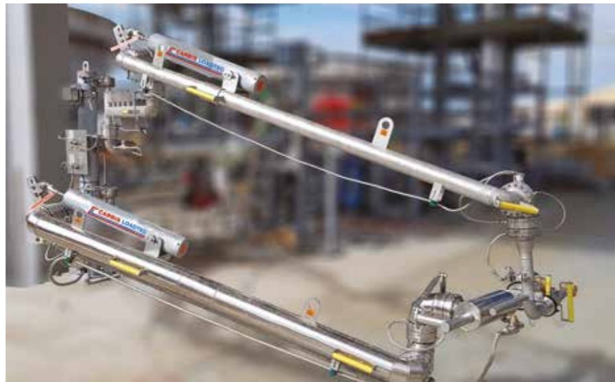
Cryoload twin bottom loading arms for use on LNG loading or unloading during SAT
