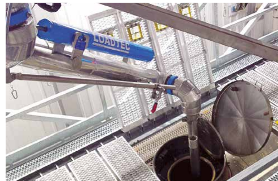
4" Heated Top loading arm for Cooking Oil - UK - Food Industry
