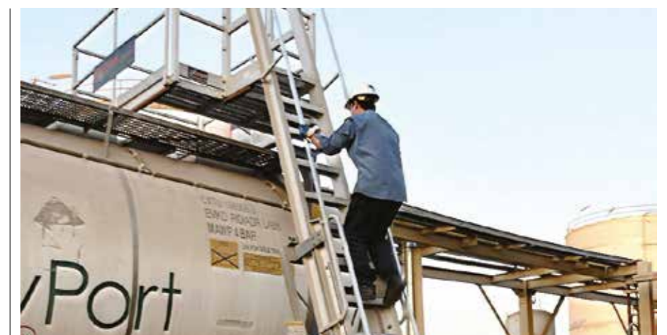
TC-10 Mobile Access Cart providing safe access to the top of container for security inspection - Saudi Arabia - Chemical Industry
