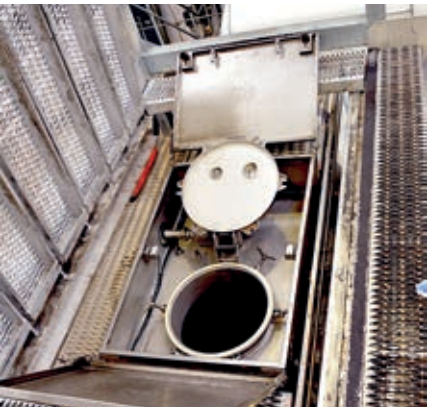
VELP panels lifted showing access to Storm Box on top of tanker
