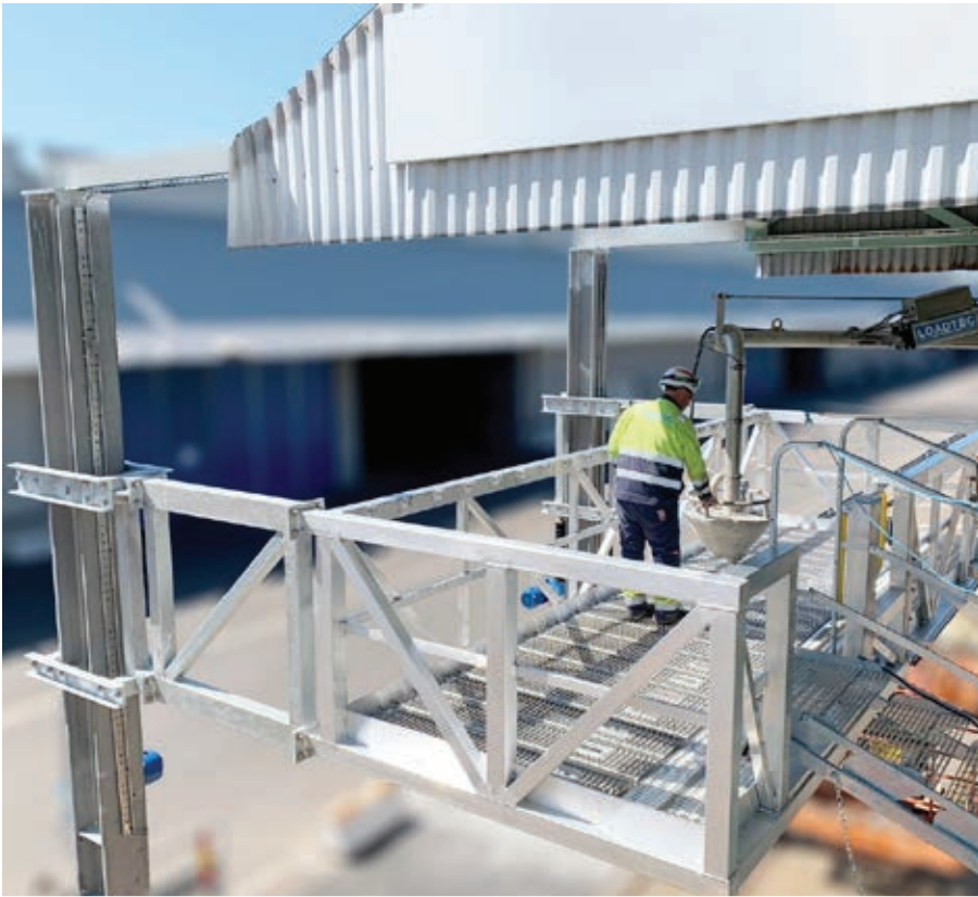
6m Electric VELP with Pneumatic top loading arm - Sweden - Chemical Industry
