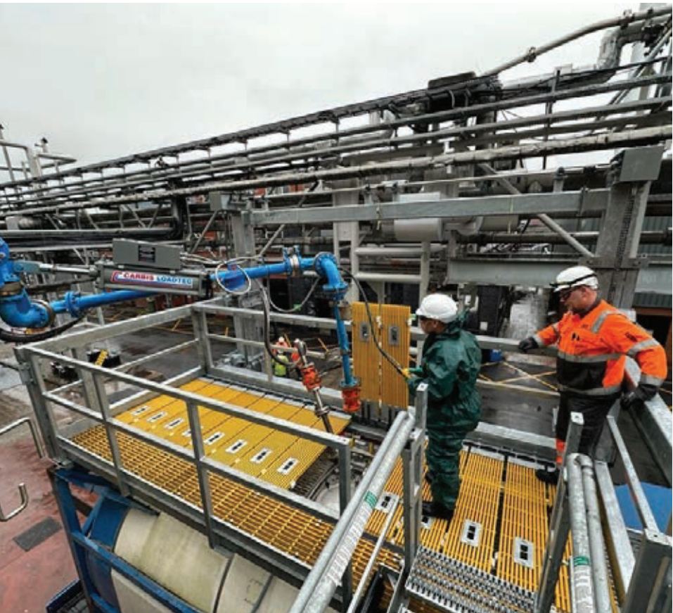
PTFE Lined Loading Arm on Vertically Elevating Platform
