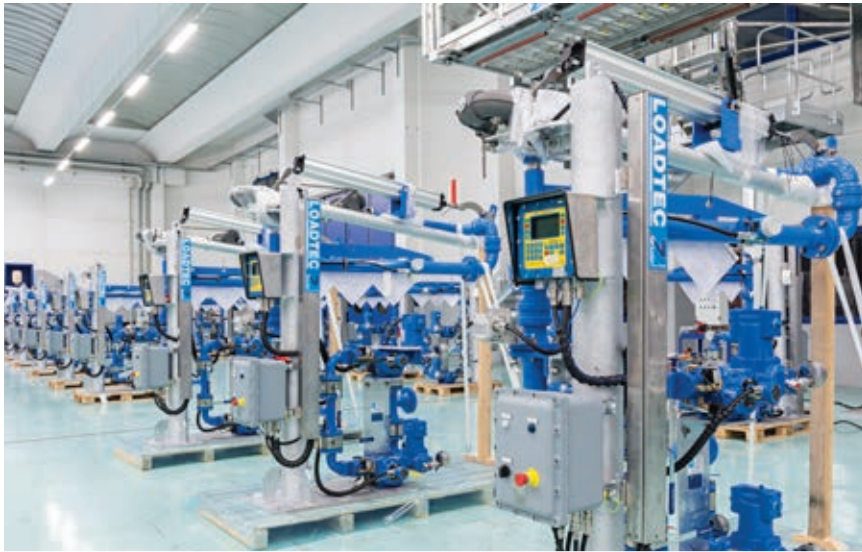
20 x Top loading skids with duty and standby metering system with batch controllers - Bangladesh - Fuels Industry
