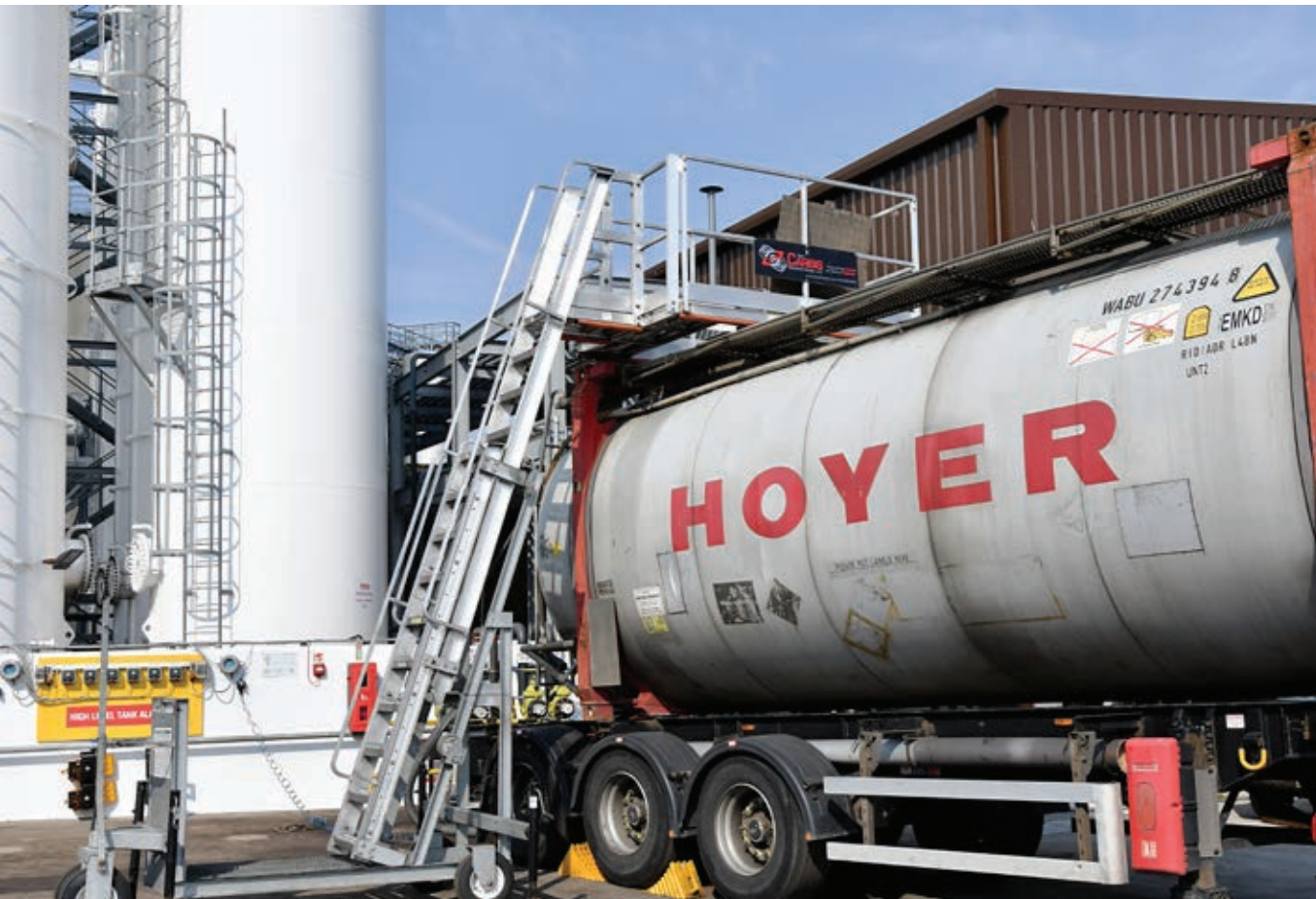
TC-10 Mobile Access Cart providing safe access to the top of an ISO container for venting during unloading - UK - Chemical Industry
