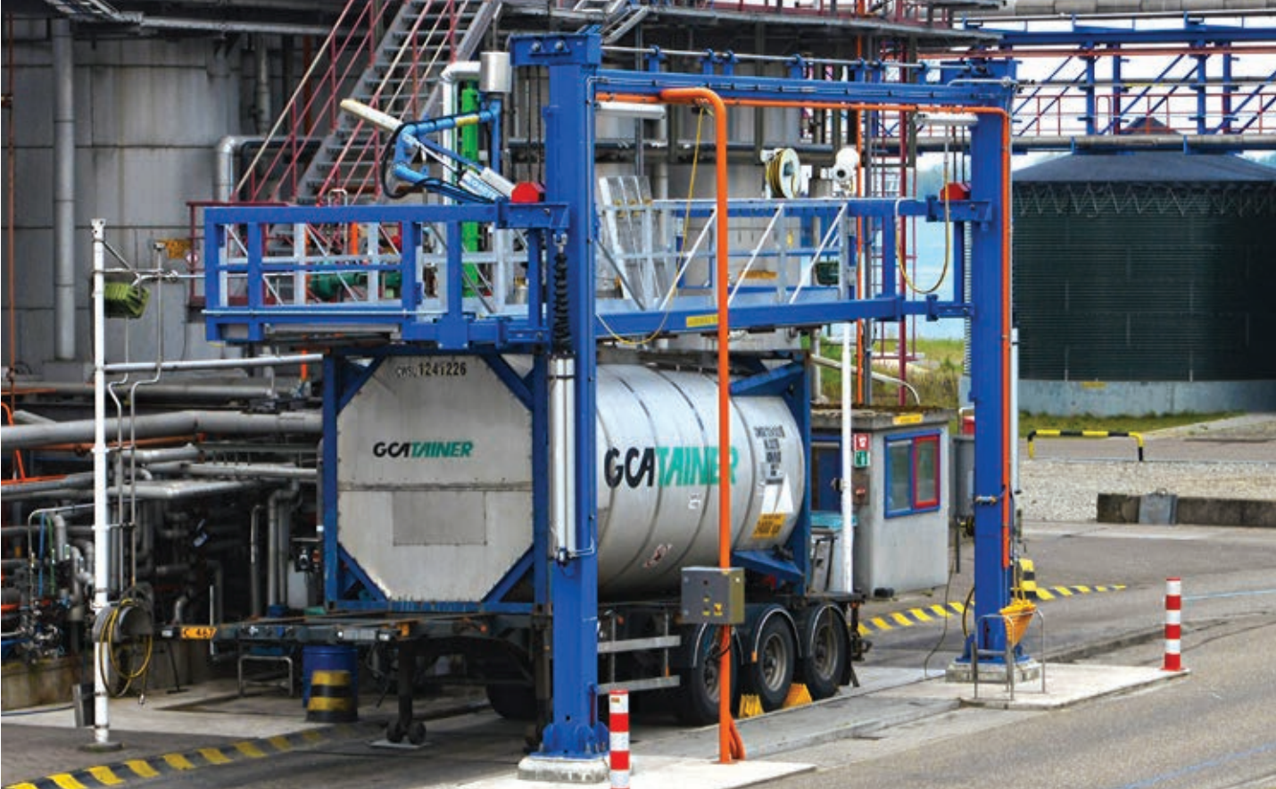
10m painted, Pneumatic VELP with pneumatic top loading arm - Netherlands - Chemical Industry
