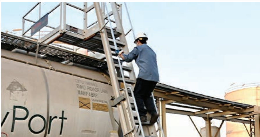
TC-10 Mobile Access Cart providing safe access to the top of container for security inspection - Saudi Arabia - Chemical Industry
