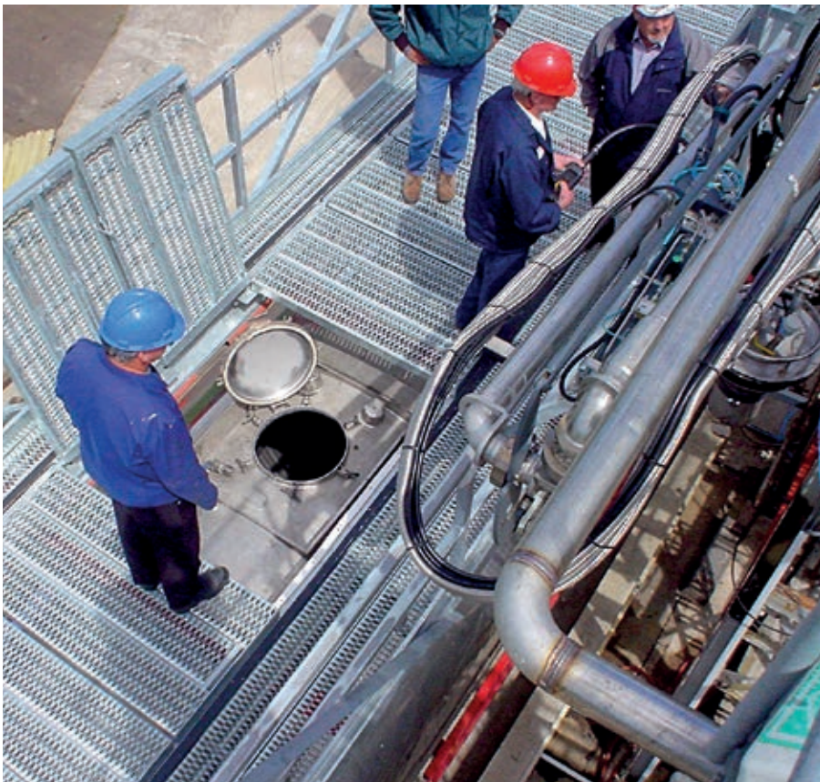
10m Hydraulic VELP with wide flip up panels providing access to tanker manlid - UK - Chemical Industry
