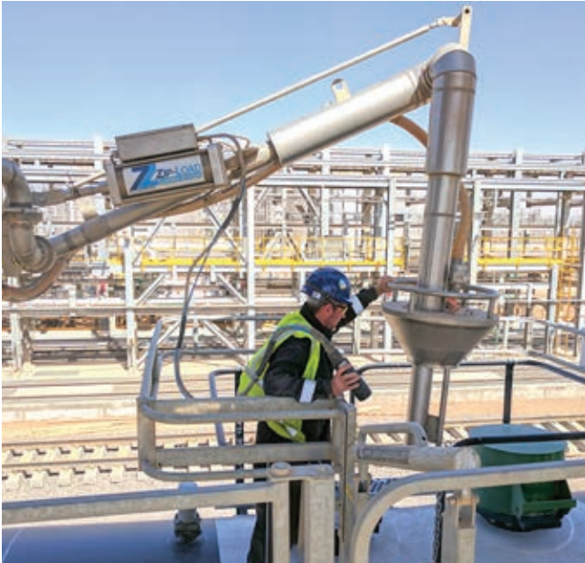
Pneumatic Top loading arm being used inside folding stair Halo cage for rail car loading - Saudi Arabia - Chemical Industry
