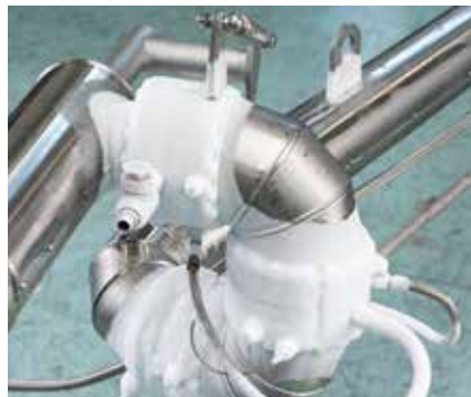
Cryoload swivels under load during FAT
