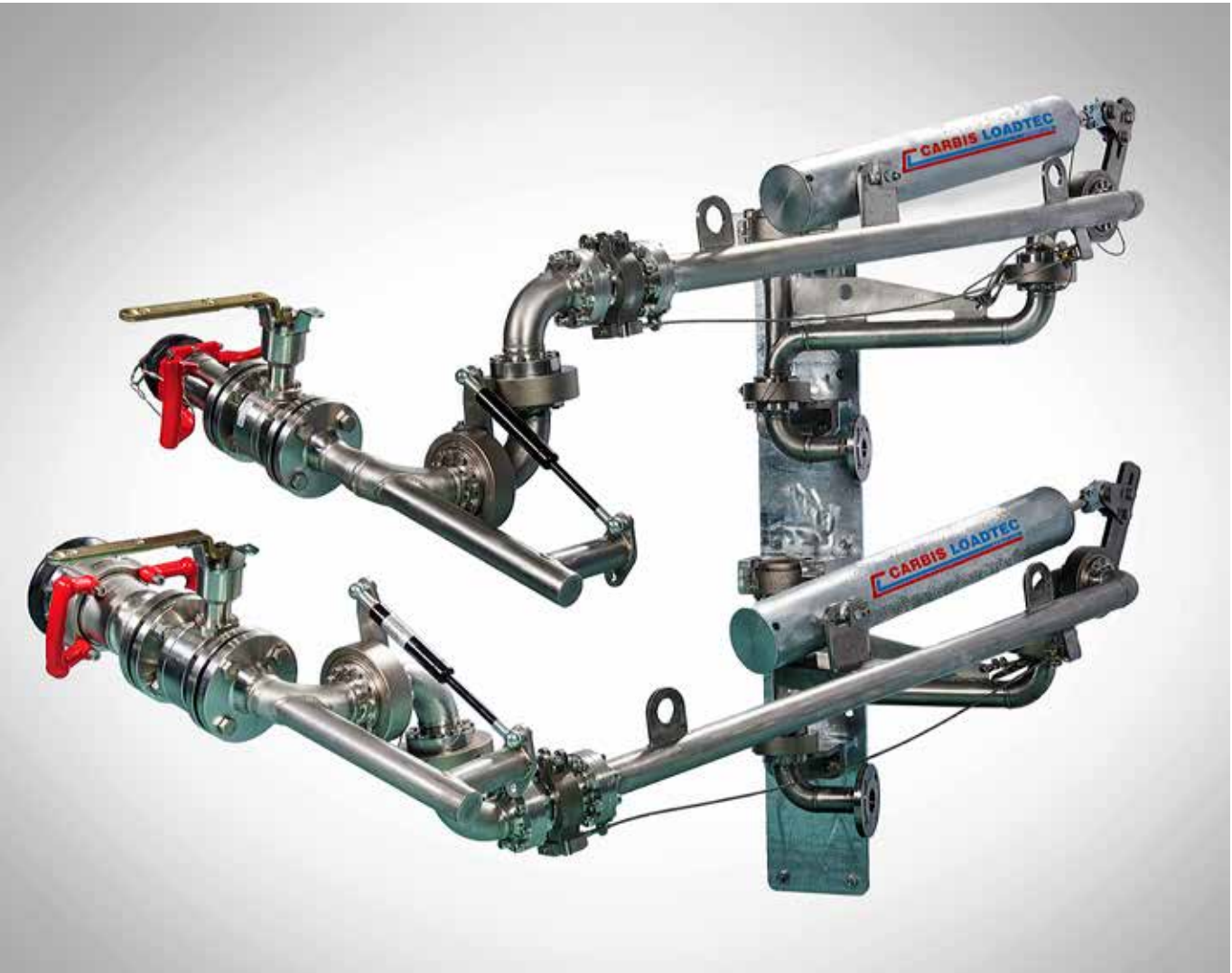
Loading and Vapour return arms mounted on a combined standpost typically for chemicals. Bottom Arm is for Product and Top Arm is for Vapour Recovery. Each with emergency release coupler, Isolation valve and Tanker Connection. - Saudi Arabia - Chemical Industry
