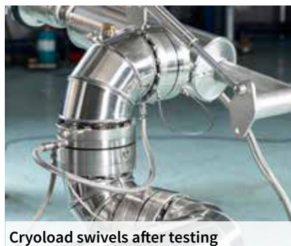
Cryoload swivels under load during FAT
