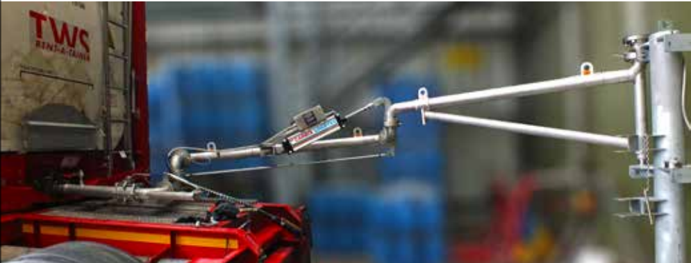
Pneumatically balanced 6 swivel Stainless Steel bottom loading arm - UK - Chemical Industry
