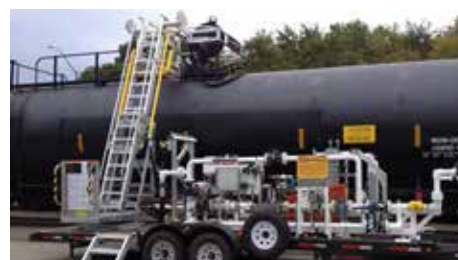
Transloading skid used to transfer product from rail cars direct to road tankers with no intermediate storage facility
